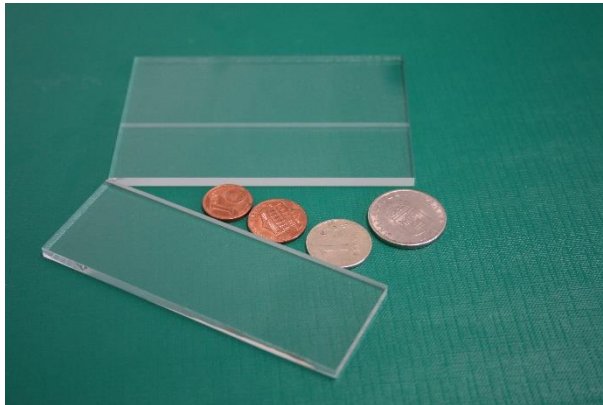
Fig.2. Glass of 4mm thickness w/ internal modifications (upper part) and after separation (lower part). Both breaking lines were processed equally in a single pass treatment.
