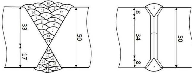
Fig. 1. (Left) SAW process; (Right) LB-SAW Hybrid process
