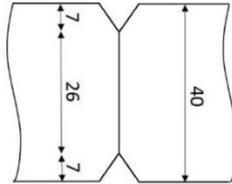
Fig. 4. Weld preparation LB-SAW Hybrid, plate thickness: 40 mm
