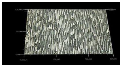
Fig. 5.8. Diffractive structure, pixel size: 4\mu\text{m} , depth 1,4\mu\text{m} , 30steps
