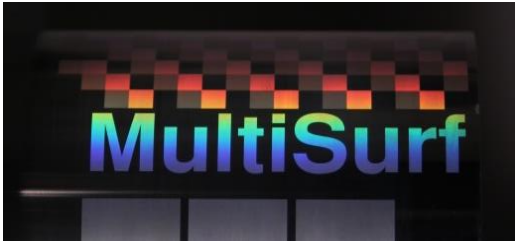
Fig. 5.9. Micro processed Logo with LIPSS structures
