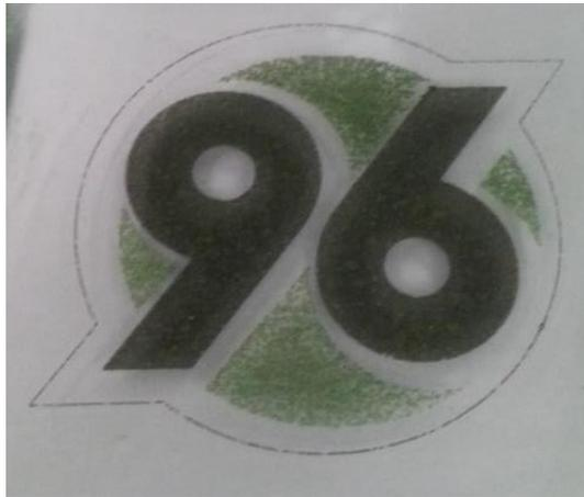
Fig. 1. Combination of laser tempering the two colors marksolid black and marksolid green, marksolid black  $f_{rep} = 10$  kHz, DC = 6 %,  $v = 600$  mm/s,  $h = 0.2$  mm; marksolid green  $f_{rep} = 10$  kHz, DC = 6 %,  $v = 700$  mm/s,  $h = 0.2$  mm;
