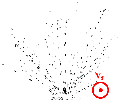
Fig. 6. Spatters resulting from welding by the means of beam oscillation with P_L = 2.5 kW, d_f = 290 \mu\text{m} , f_{x,y} = 100 Hz, w_{x,y} = 1.5 mm, v_F = 6 m/min, l = 200 mm.
