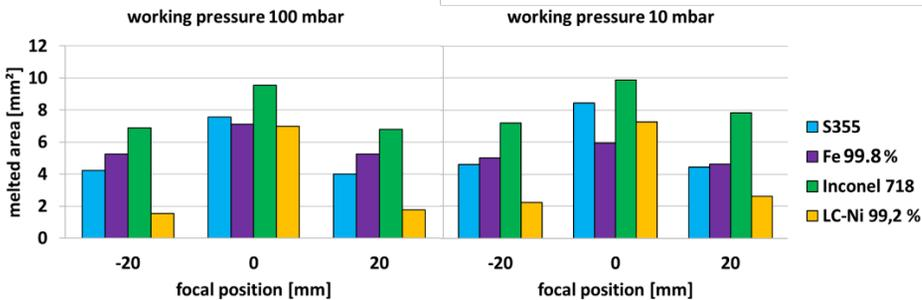
Fig. 3. Melted area of investigated cross sections at working pressure of 100 mbar (left) and 10 mbar (right)
