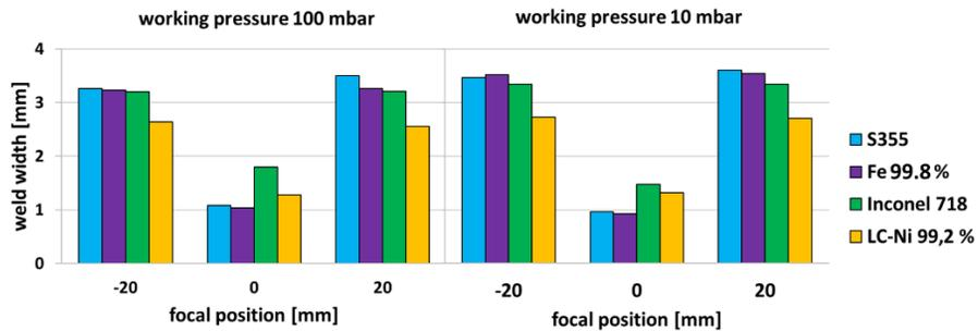
Fig. 2. Weld widths of investigated cross sections at working pressure of 100 mbar (left) and 10 mbar (right)
