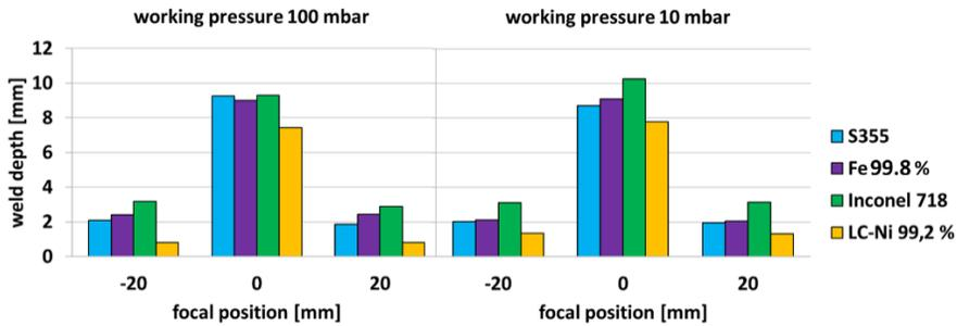
Fig. 1. Weld depths of investigated cross sections at working pressure of 100 mbar (left) and 10 mbar (right)
