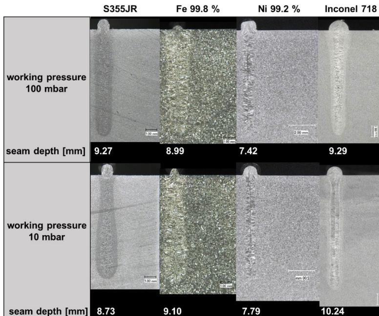
Fig. 4. Cross sections of selected weld seams at surface focus with working pressure 100 mbar (top) and 10 mbar (bottom)
