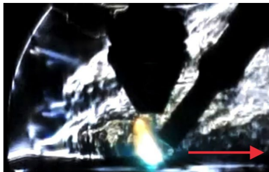
Fig. 3. Schlieren image of gas flow during laser-TIG welding. Red arrow - welding direction
