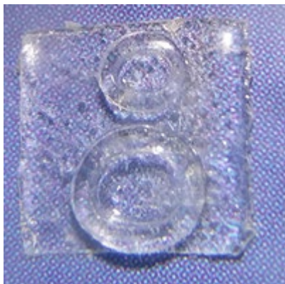
Fig. 3. 3D printed part with Selective Laser Baking (SLB) technique.
