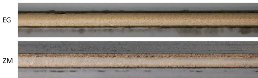
Fig. 4. Exemplary surface appearance of laser brazed joints on EG and ZM coated steel at outer joining radii of 2.6 mm
