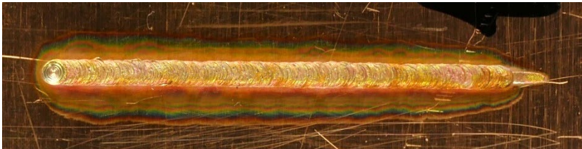
Fig. 7. Weld bead surface of an overlap weld (1 mm copper on 2 mm copper sheet), showing a homogeneous weld bead surface with spatter free process ( P_{\text{blue}}=1000\text{W} , P_{\text{IR}}=3000\text{W} , v=2\text{ m/min} )
