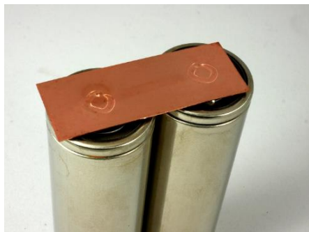
Fig. 5: Two welded 21700 cylindrical battery cells with the LDMblue1000-100 ( v=75 \text{ mm/s} , 450 nm wavelength)
