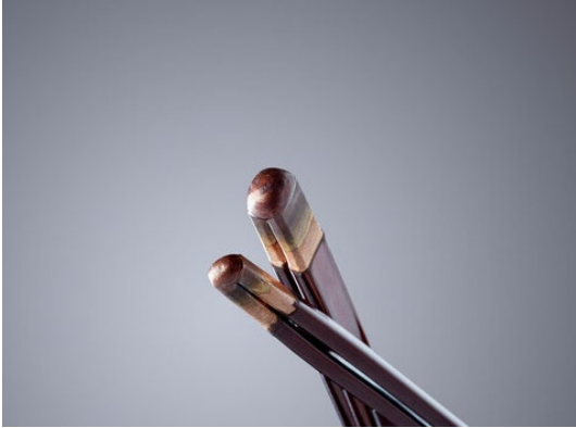
Fig. 1. Samples of different types of hairpins. The front ends are laser welded [TRUMPF].
