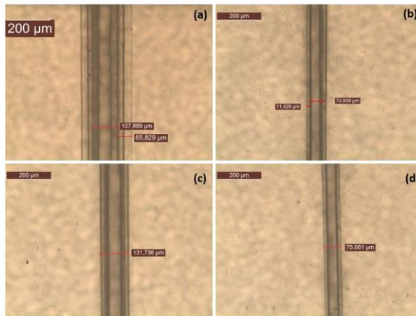
Fig. 8. Optical microscope image of 5 mil thick PET sample cut with 515 nm femtosecond pulses in (a) single scan mode at 1 MHz repetition rate (b) multi-scan mode at 1 MHz repetition rate; (c) single scan mode at 2 MHz repetition rate (d) multi-scan mode at 2 MHz repetition rate.
