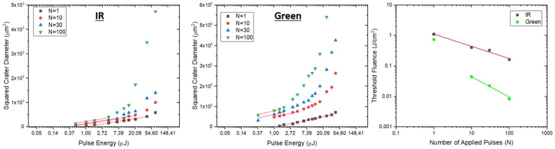
Fig. 2. Plot of squared crater diameters versus the pulse energy for different number of applied laser pulses on a PET sample when irradiated with (a) IR (1030 nm) fs laser pulses (b) green (515 nm) fs laser pulses; (c) Plot of threshold fluence versus number of pulses, N of a PET sample for IR and green wavelengths.
