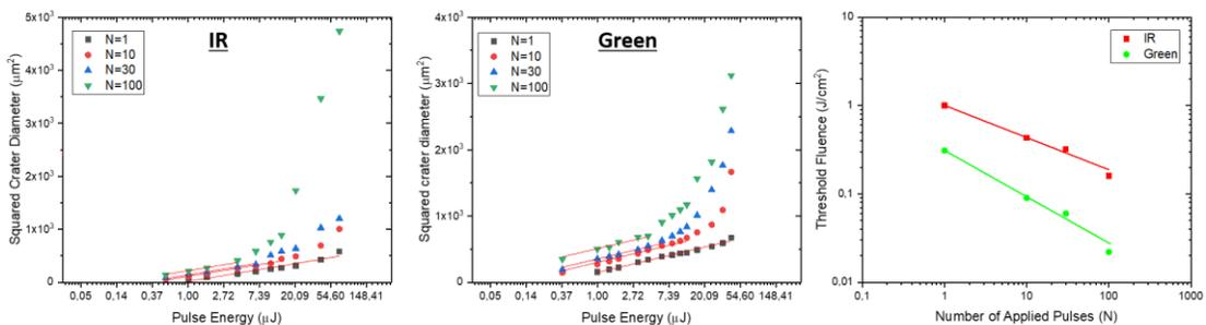
Fig. 1. Plot of squared crater diameters versus the pulse energy for different number of applied laser pulses on a polyimide sample when irradiated with (a) IR (1030 nm) fs laser pulses (b) green (515 nm) fs laser pulses at 1 MHz repetition rate; (c) Plot of threshold fluence versus number of pulses,  $N$  of a polyimide sample for IR and green wavelengths with laser running at 1 MHz repetition rate.
