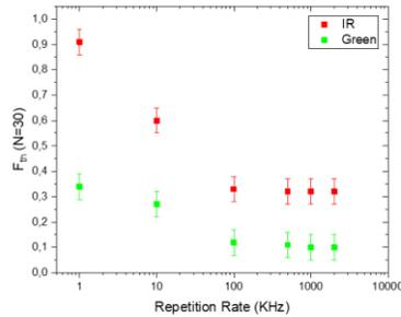
Fig. 3. Threshold Fluence values for 30 pulses versus the repetition rate on a polyimide sample when irradiated with 1030 nm and 515 nm laser pulses
