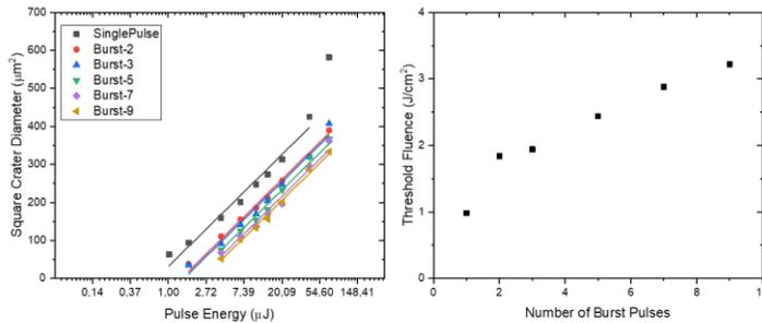
Fig. 4. (a) Plot of squared crater diameters versus the pulse energy for different number of burst pulses on a polyimide sample when irradiated with IR (1030 nm) fs laser pulses at 1 MHz repetition rate; (b) Threshold Fluence values versus the number of burst pulses on a polyimide sample when irradiated with IR (1030 nm) fs laser pulses at 1 MHz repetition rate.
