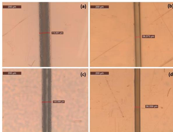
Fig. 6. Optical microscope image of 5 mil thick polyimide sample cut with 515 nm femtosecond pulses in (a) single scan mode at 1 MHz repetition rate (b) multi-scan mode at 1 MHz repetition rate; (c) single scan mode at 2 MHz repetition rate (d) multi-scan mode at 2 MHz repetition rate.
