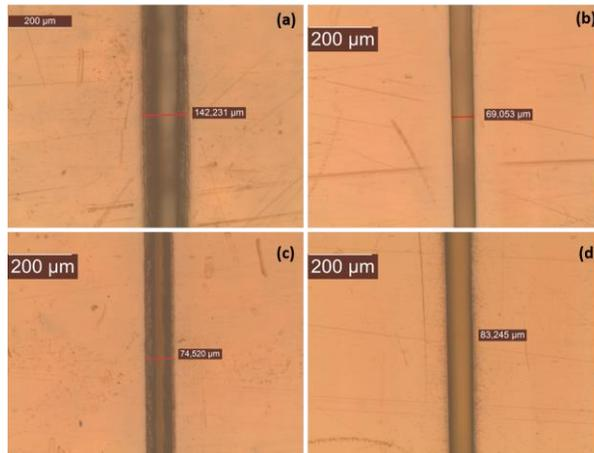
Fig. 5. Optical microscope image of 5 mil thick polyimide sample cut with 1030 nm femtosecond pulses in (a) single scan mode at 1 MHz repetition rate (b) multi-scan mode at 1 MHz repetition rate; (c) single scan mode at 2 MHz repetition rate (d) multi-scan mode at 2 MHz repetition rate.
