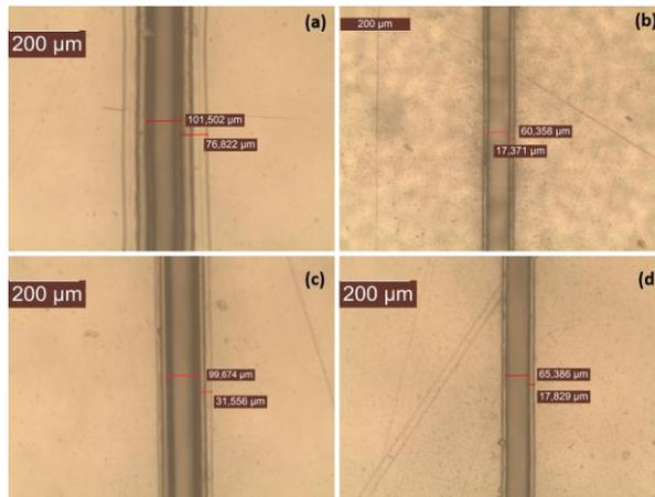
Fig. 7. Optical microscope images of 5 mil thick PET sample cut with 1030 nm femtosecond pulses in (a) single scan mode at 1 MHz repetition rate (b) multi-scan mode at 1 MHz repetition rate; (c) single scan mode at 2 MHz repetition rate (d) multi-scan mode at 2 MHz repetition rate.
