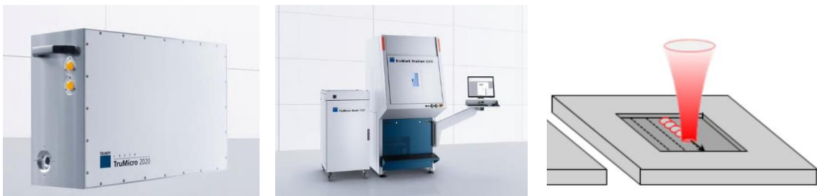
Fig. 2. (a) TruMicro Series 2000. (b) TruLaser Station 5005. (c) Ablation of small pockets to evaluate ablation efficiency and surface quality depending on the applied laser parameters.
