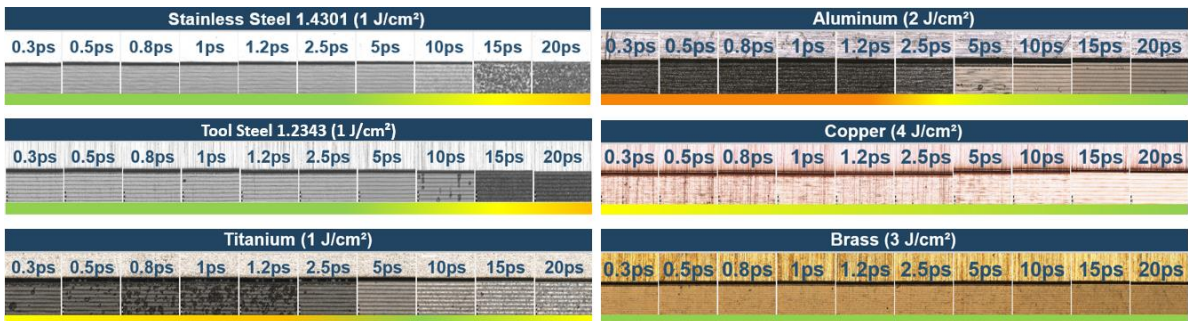
Fig. 5. Machined surface quality trends for different pulse durations and optimum fluence levels. The scan speed and repetition rate varied depending on the material. The number of repetitions was adjusted for an ablation depth of at least 50 μm. Each image shows the raw material in the top half and the machined surface in the bottom half. For the two steel grades, best results are observed for shorter pulse durations, whereas for aluminum and titanium, longer pulse durations can be beneficial regarding surface quality. On copper and brass, only small changes in surface quality are seen in the studied parameter range.
