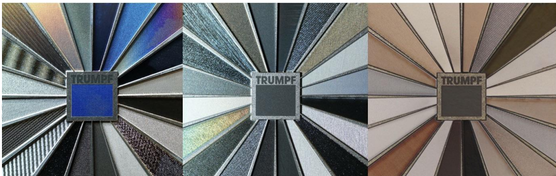
Fig. 1. High-quality engravings in (a) titanium, (b) stainless steel (DIN EN 1.4404) and (c) copper. Highly flexible laser systems can address all kind of surface qualities by tailoring the temporal energy deposition on several orders of magnitude from a fs- to \mu s-timescale.
