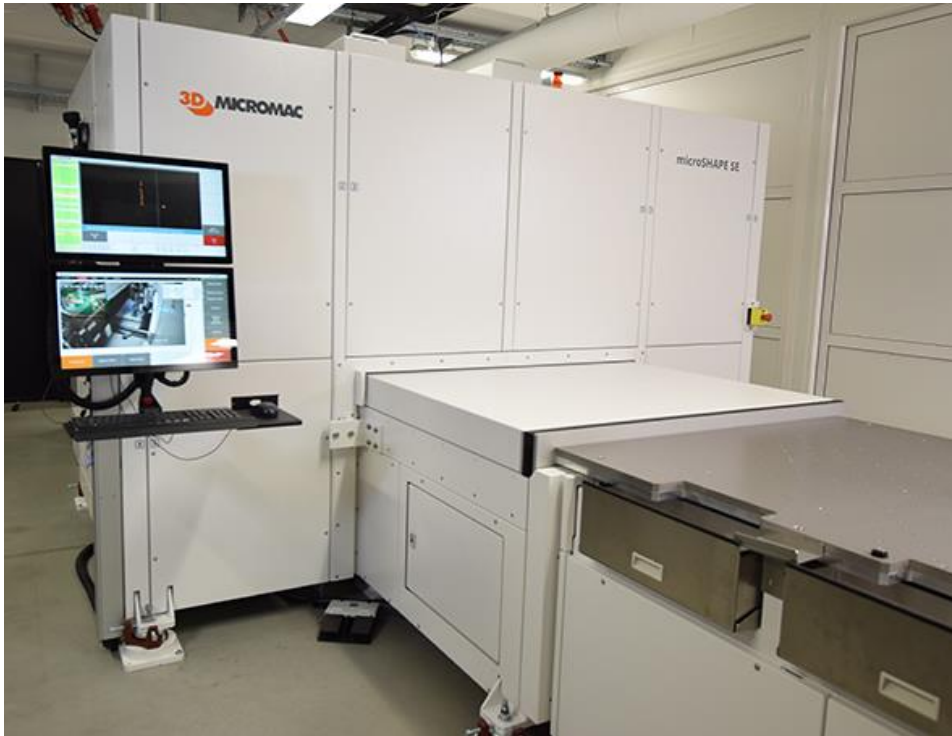
Fig. 6. Example of Laser System microSHAPE SE, dedicated for manual loading or line integration in sheet-to-sheet or roll-to sheet process flows
