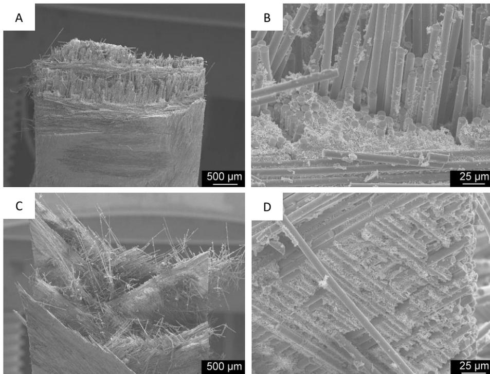
Fig. 6. SEM micrographs of the fracture surface after tensile test; (A)  $0^\circ/90^\circ$ , (B) higher magnification of (A); (C)  $+60^\circ/-60^\circ$ ; (D) higher magnification of (C)
