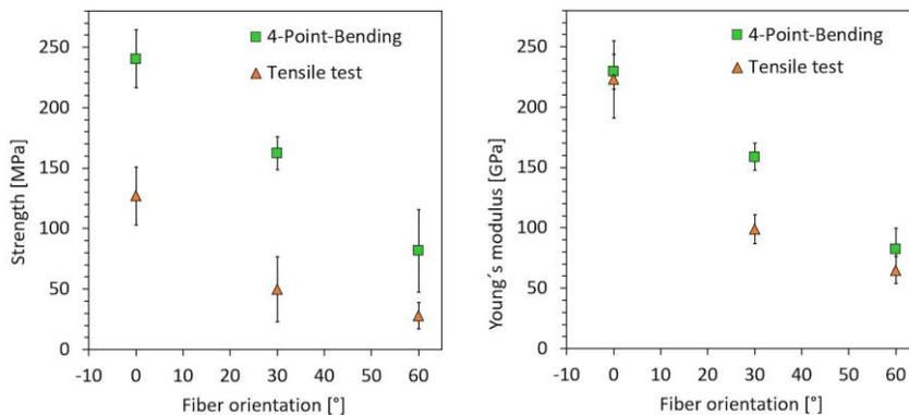
Fig. 5. Mechanical properties of FAST/SPS specimens depending on fiber orientation at room temperature; (left) Tensile strength, (right) Young's modulus
