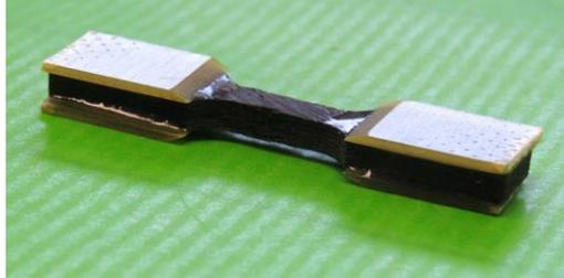
Fig. 2. Tensile test specimen with glass fiber reinforced polymer pads glued to the shoulders to reduce stress gradients from clamping
