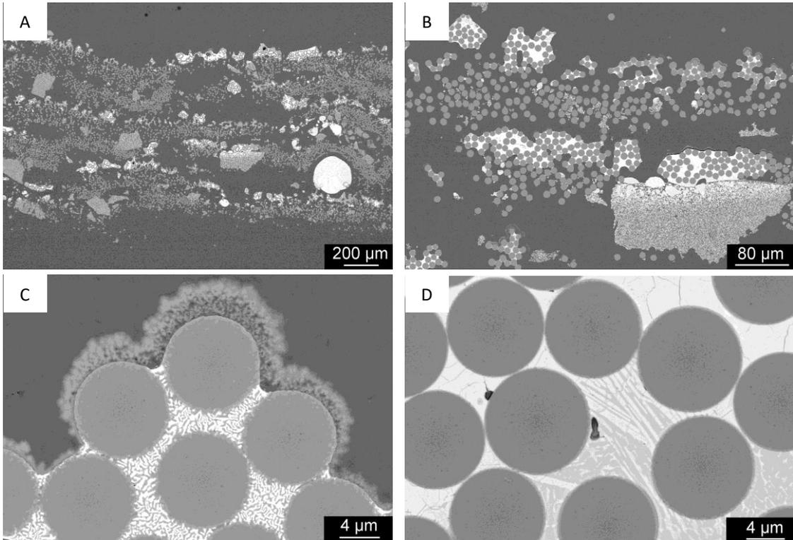
Fig. 3. SEM pictures of the microstructure after Laser-treatment; (A) complete cross-section, (B) magnified middle-section; (C) overheated region, (D) aimed microstructure
