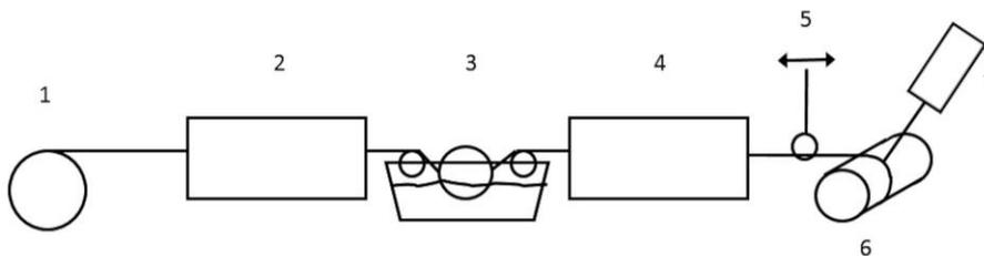
Fig. 1. Schematic drawing of the manufacturing process; 1: Fiber-roll, 2: Desizing, 3: Suspension coating, 4: Drying, 5: Fiber placement, 6: Rotating mandrel, 7: Laser [8]
