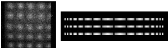
Fig. 2. Examples of DOEs with (left) a squared array of dots and (right) a modulated light intensity distribution in three parallel lines
