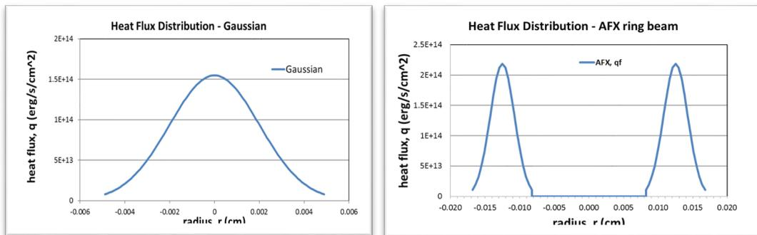
Fig. 2. Heat flux profile distributions for a Gaussian and a ring beam
