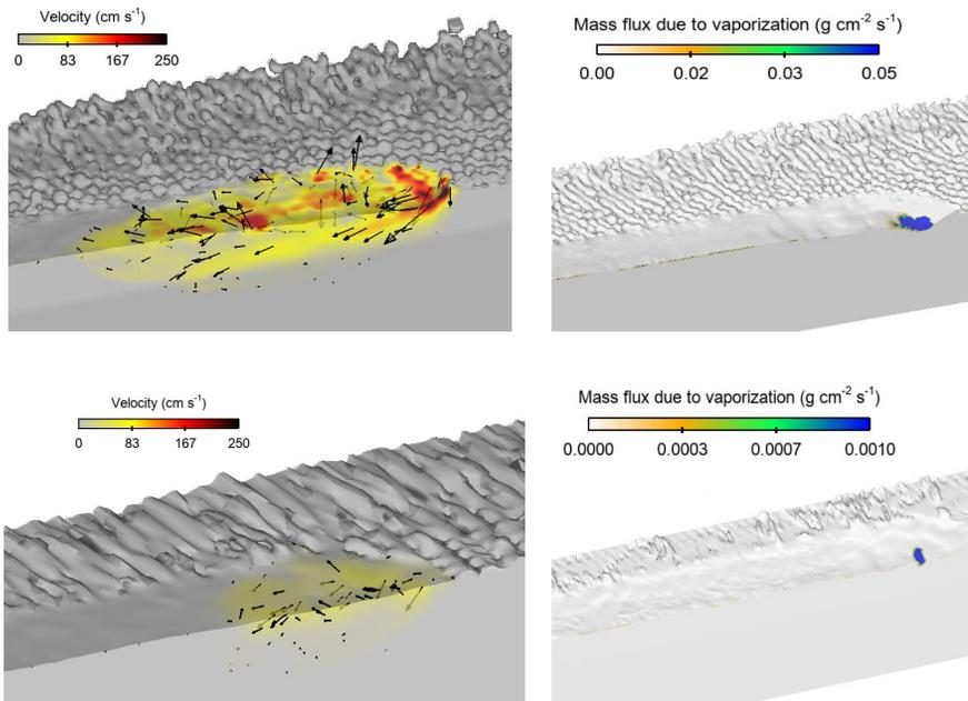
Fig. 4. Melt pool velocities and mass flux due to phase change (Gaussian – top and Ring beam – bottom)
