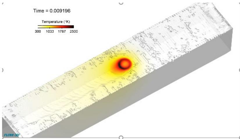
Fig. 3. A melt pool simulation showing temperature profiles in a ring beam simulation
