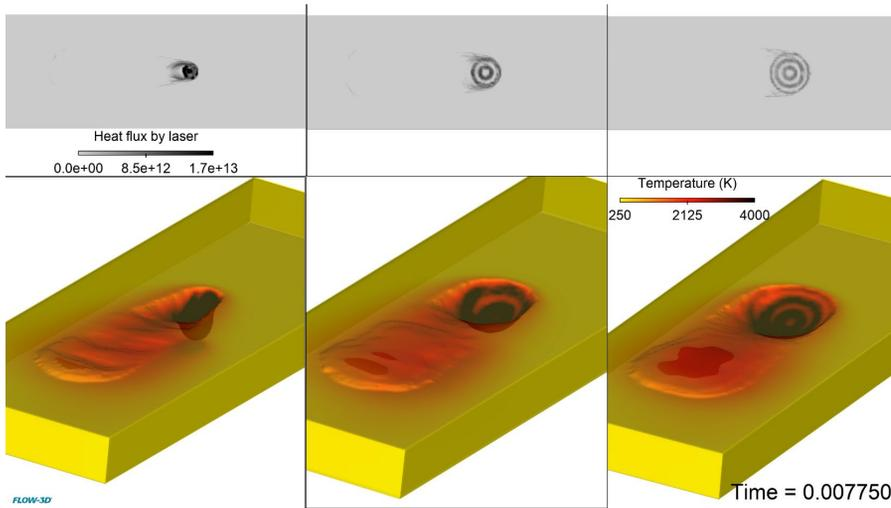
Fig. 1. Melt pool dynamics for different laser beam shapes
