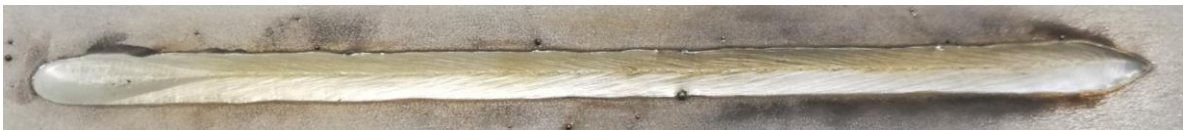
Fig. 7. Welding seam at 7kW
