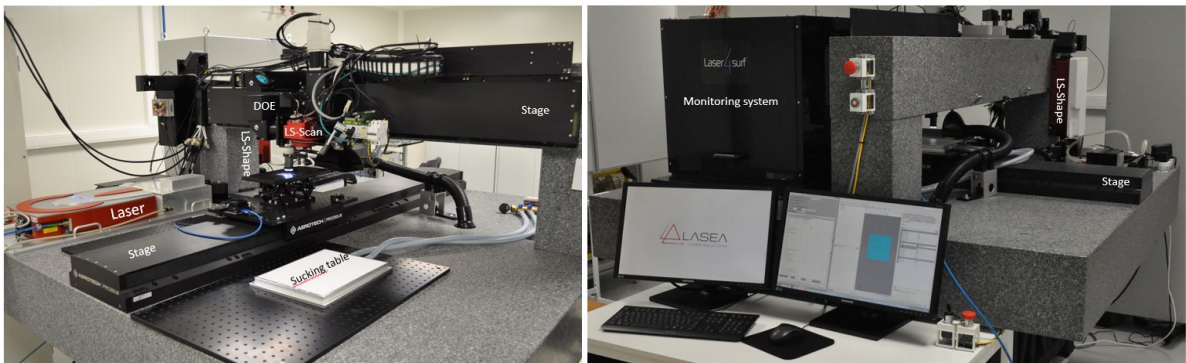
Fig. 1. (a) front view of the laser workstation without the monitoring system; (b) side view of the laser workstation with the monitoring system integrated
