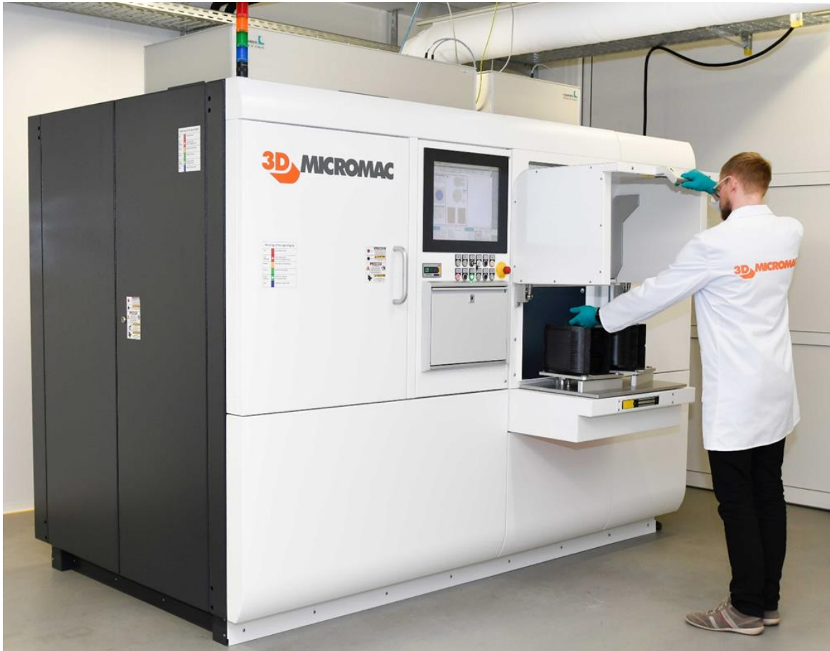
Fig. 4. microVEGA xMR selective laser annealing system for monolithic magnetic sensor formation.
