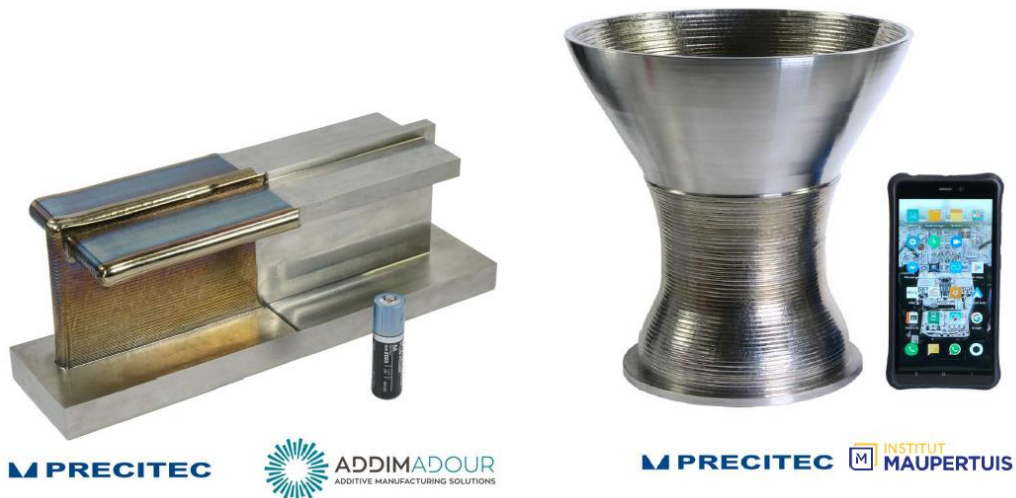
Fig. 7. DED-LB wire part printed with TA6V
