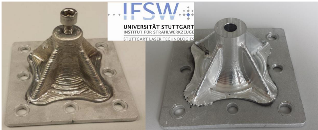
Fig. 6. OCT controlled DED-LB wire part made of AlMg5
