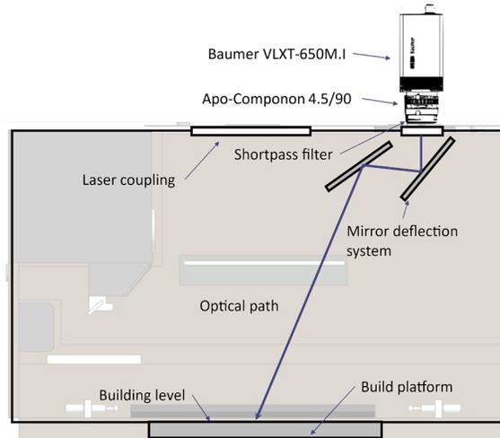
Fig. 2. Schematic experimental setup of SLM 280HL for position detection of objects
