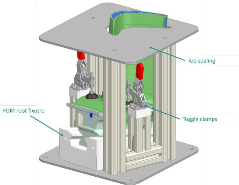
Fig. 2. Fixturing system for turbine blade including top sealing to prevent powder sag (root pixelated due to non-disclosure)
