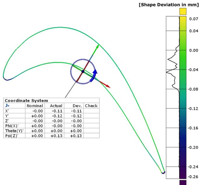
Fig. 4. Evaluation of the shape and position deviation of the hybrid repair process
