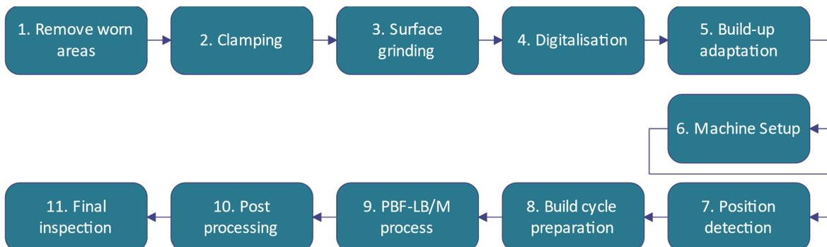
Fig. 1. Process chain of hybrid repair process using PBF-LB/M
