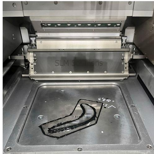
Fig. 3. (a) installation of mounted fixturing system within SLM 280HL machine; (b) sealed turbine blade leveled during pre processing (root and cooling channels pixelated due to non-disclosure)
