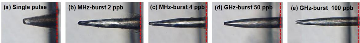
Fig. 1. Microscope images of drilled holes after 100 ms drilling time with an energy of 200  $\mu\text{J}$  distributed on (a) Single pulses; (b) MHz-bursts with 2 pulses per burst; (c) MHz-bursts with 4 pulses per burst; (d) GHz-bursts with 50 pulses per burst; (e) GHz-bursts with 100 pulses per burst.
