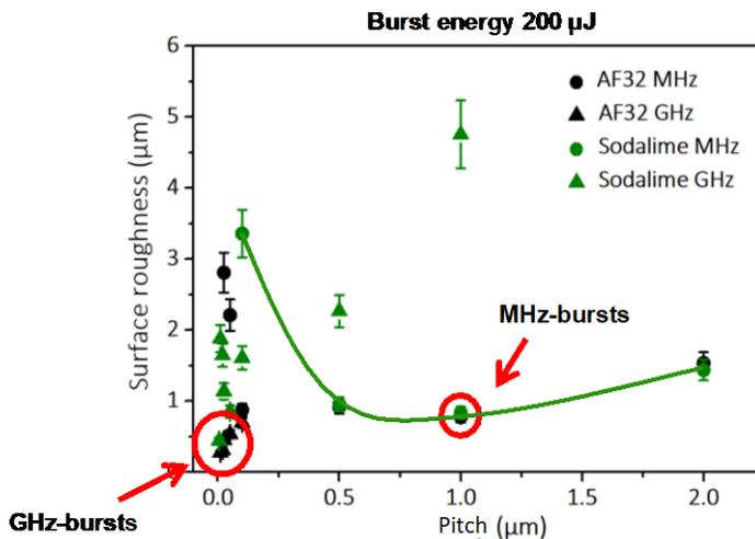
Fig. 3. Surface quality  $S_a$  as a function of the pitch in sodalime (green symbols) and AF32 (black symbols) for GHz-bursts of 50 pulses per burst (triangles) and MHz-bursts of 4 pulses per burst (dots) at  $200 \mu\text{J}$  burst energy for both regimes.
