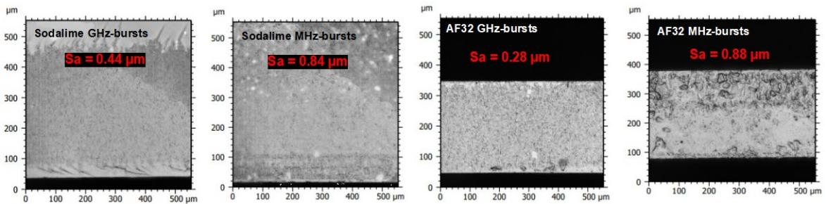
Fig. 4. Profilometer images of the cutting planes with an energy of 200  $\mu\text{J}$  in GHz-burst mode with 50 pulses per burst and in MHz-burst mode with 4 pulses per burst. The pitches are 0.05  $\mu\text{m}$  in GHz-burst mode and 1  $\mu\text{m}$  in MHz-burst mode, respectively. Laser comes from the bottom.
