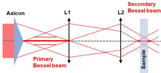
Fig. 2. Schematic drawing of the Bessel beam formation by an axicon into a primary Bessel beam with subsequent imaging into a secondary Bessel beam with smaller dimensions.
