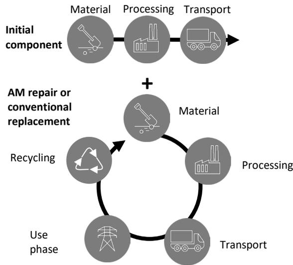
Fig. 2. System boundary of the CO<sub>2</sub>e assessment: Two stages. 1<sup>st</sup>, upper: Initial component. 2<sup>nd</sup>, lower: Replacement component. The second stage can be either conventional 1-to-1 replacement or AM-repair.
