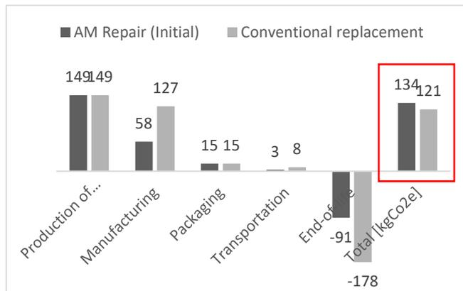
Fig. 3. Initial results of the comparative study of CO<sub>2</sub>e: The conventional replacement emits 13 kgCO<sub>2</sub>e less than the AM-repair.
