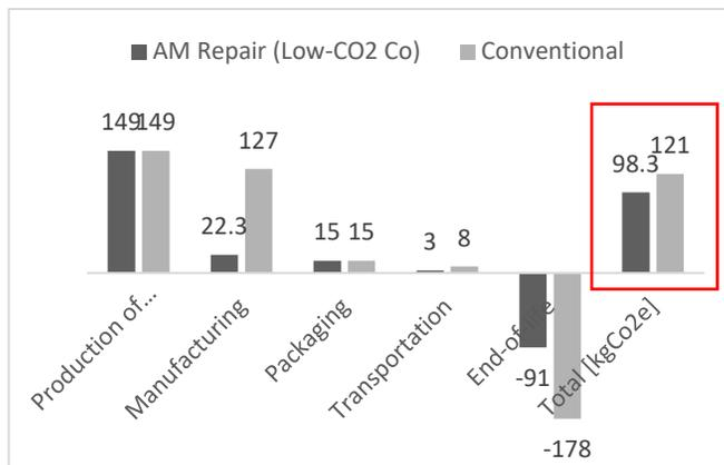
Fig. 5. Assuming “least-impact cobalt (Co) mining results in 23 less kgCO<sub>2</sub>e for the AM remanufacturing.
