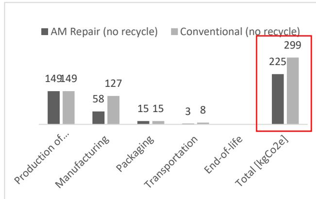
Fig. 4. Assuming no recycling at the end-of-life results in 74 kgCO<sub>2</sub>e less for the AM remanufactured component set.
