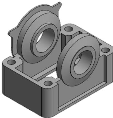
Fig. 1. Simplified CAD-model of the bearing bridge subject to the carbon footprint study (pin bolt not shown).
