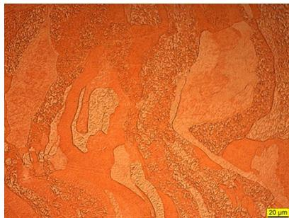
Fig. 2. A microsection through pure copper printed with > 99.9% density.
