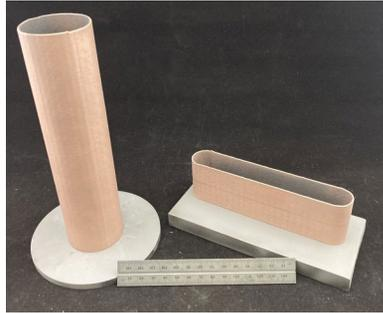
Fig. 4. LMD of GR Cop 42 with Green printed at Fraunhofer ILT (Plymouth, Michigan).
