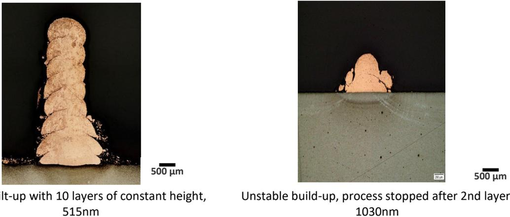
Fig. 3. Comparison of Green and IR deposits for "fillet" structure with CuCrZr powder.
