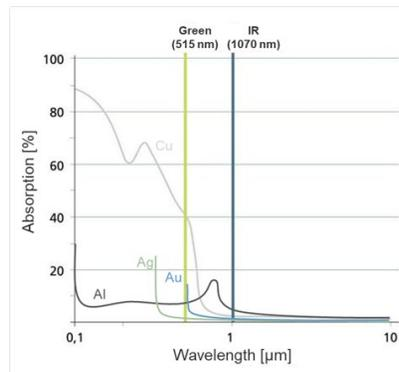
Fig. 1. Comparison of Green and IR laser wavelengths vs absorption
