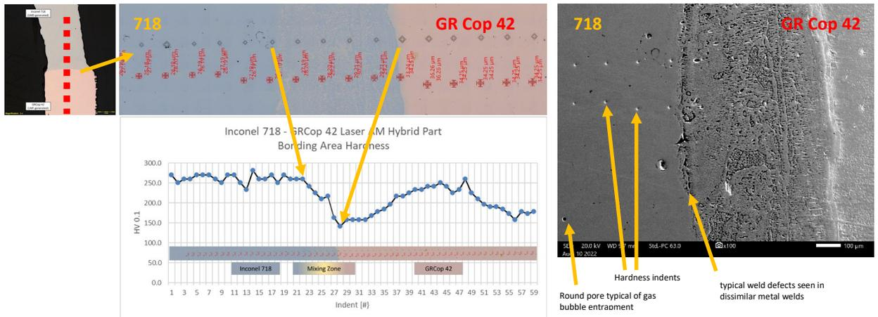
Fig. 5. Interface zone showing typical defects seen in dissimilar weld joints and hardness drops.
