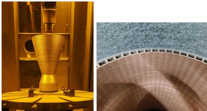
Fig. 7. Bi-metallic GR Cop 42- 625 structure build by RPMI using TRUMPF green lasers.
