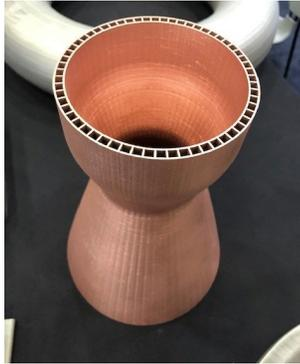
Fig. 6. Initial GR Cop 42 structure build by RPMI using a TRUMPF green laser optic.
