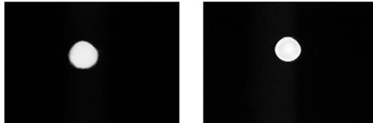
Fig. 15. Nickel,  $t=6$  mm; Entry diameter  $168\mu\text{m}$  (left); Exit diameter  $148\mu\text{m}$  (right)
