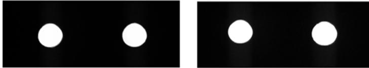
Fig. 14. Nickel,  $t=6$  mm; Entry diameter  $278\mu\text{m}$  (left); Exit diameter  $278\mu\text{m}$  (right)
