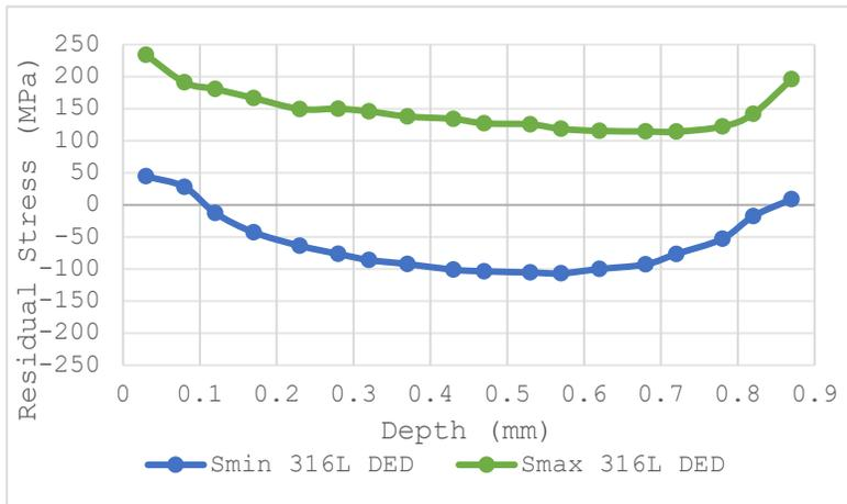
Fig. 3. Residual stress profile of the DED sample as built.
