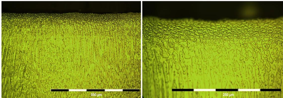
Fig. 2. Effect of the LSP treatment on the microstructure of the DED consolidated material. More general view to the left, detailed view to the right
