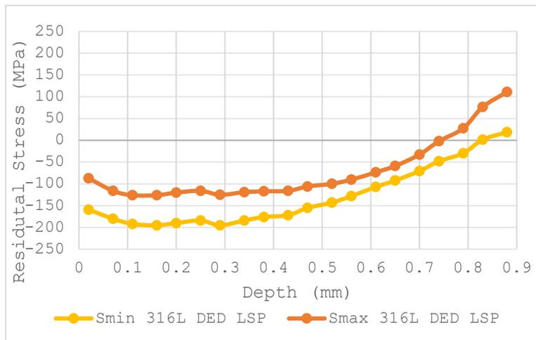
Fig. 4. Beneficial compressive residual stress profile after the treatment of the surface of the DED sample.
