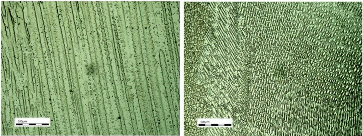
Fig. 1. Columnar growth pattern of the consolidated material (left) and cellular growth pa.
