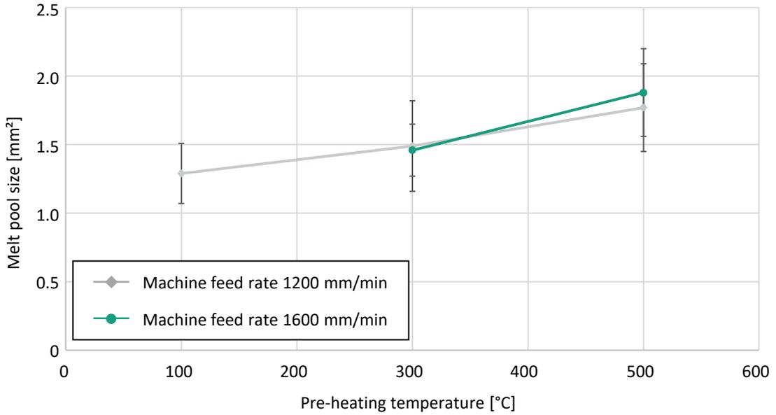
Fig. 5. Melt pool size in dependence on the pre-heating temperature and the machine feed rate
