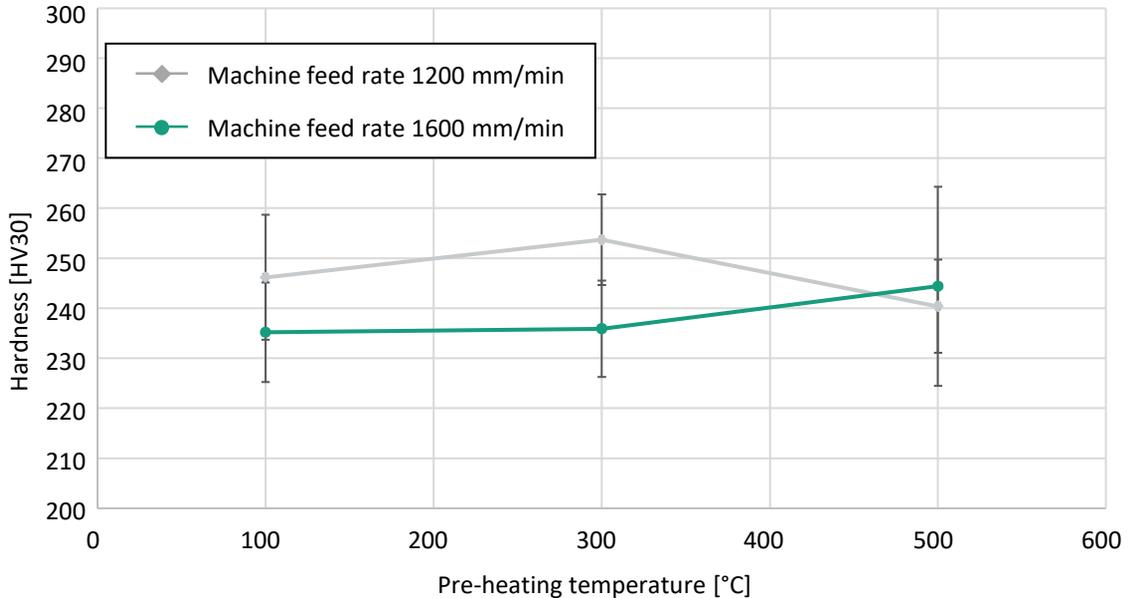
Fig. 7. Hardness in dependence on pre-heating temperature and machine feed rate
