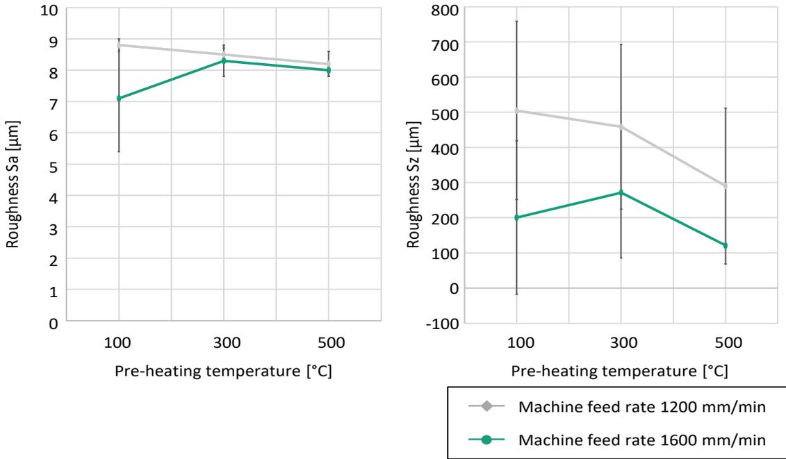
Fig. 6: Roughness Sa and Sz in dependence on pre-heating temperature and machine feed rate
