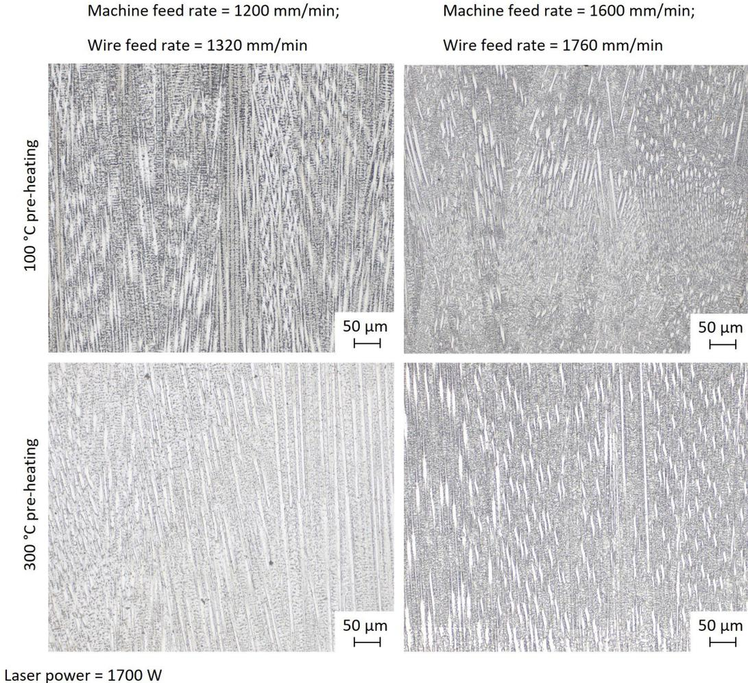
Fig. 3. Microstructure of IN718 in dependence on the pre-heating temperatures and machine feed rates
