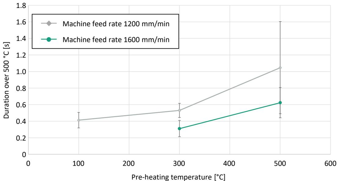
Fig.4. Duration of segment temperature over 500°C in dependence on pre-heating temperature and machine feed rate
