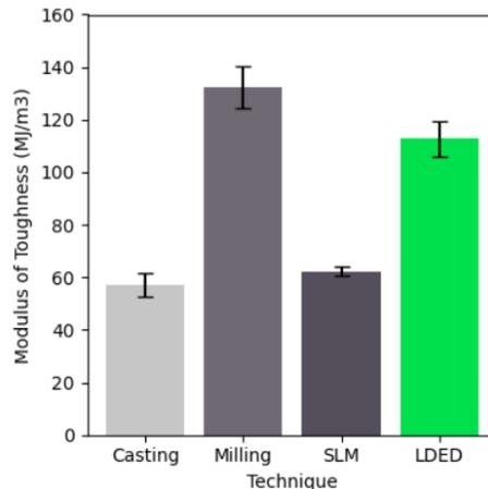
Fig. 3. Modulus of toughness of all materials obtained by casting, milling from disk, SLM and LDED.
