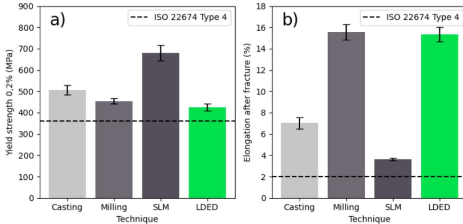
Fig. 2. Yield strength 0,2% (a) and Elongation after fracture; (b) of all materials obtained by casting, milling from disk, SLM and LDED.
