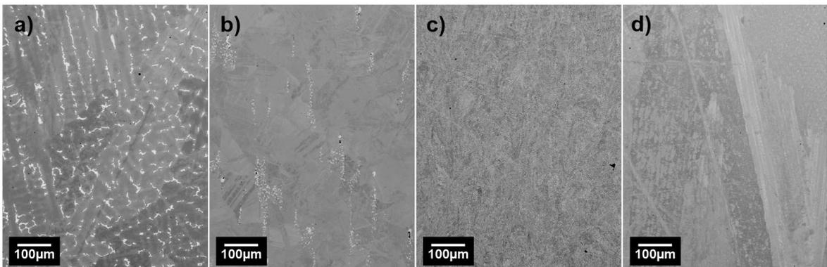
Fig. 1. SEM micrographs displaying a longitudinal section of each fabrication technique: (a) casting; (b) milling from disk; (c) SLM; and (d) LDED.
