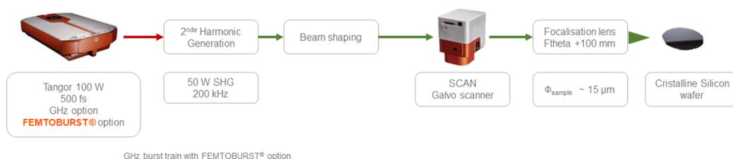
Fig. 1. Schematic representation of the laser system used for GHz ablation at 515 nm.
