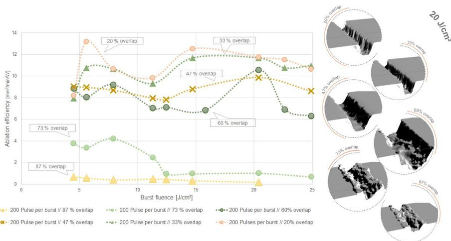
Fig. 2. Line scribing obtained with 515 nm GHz bursts on silicon. The effect of the pulse overlap is shown both on the ablation efficiency and on the scribing quality.
