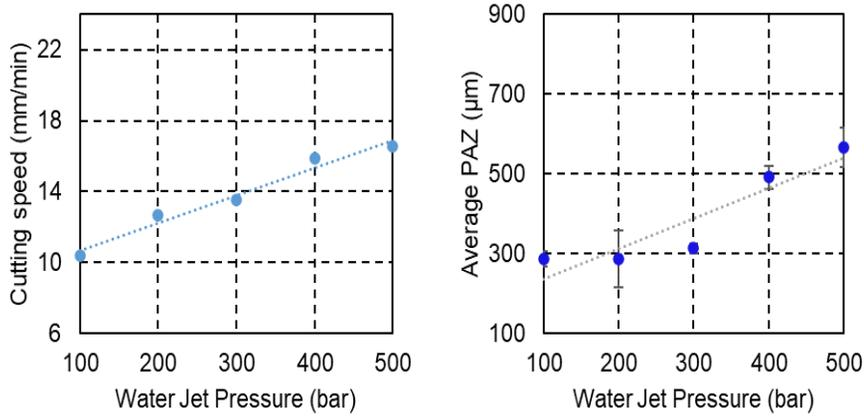
Fig. 2. Effect of water jet pressure on cutting performance.
