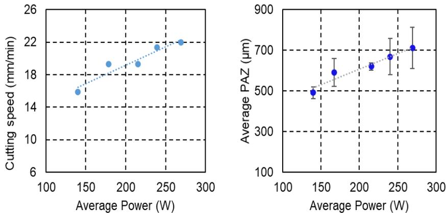
Fig. 3. Effect of average power on cutting performance.
